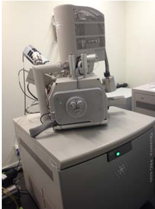
Figure 5.13: Photograph of the FEI Quanta 650 FEG SEM equipment used in this work.
