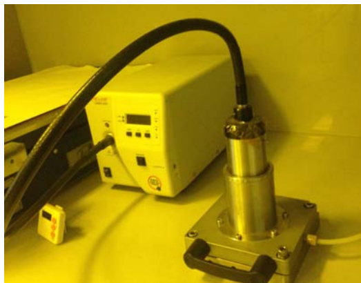
Figure 5.8: Photograph of the UV-assisted NIL setup
