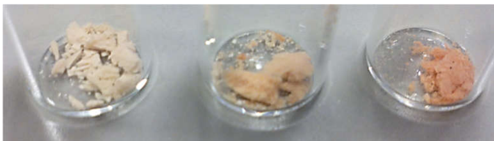
Figure 4.74 Image of lyophilized biomass coming from three different tanks, from a three-stage CSTR. From left to right, first, second and third bioreactor biomass, respectively. The last step show biomass with a strong orange colour.
