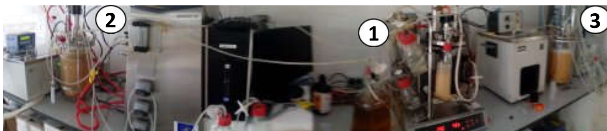
Figure 4.73 Illustration of a triple tank system used in this study. Number 1 shows the first bioreactor with a volume of 1.7 L, and number 2 and 3 indicate the polishing bioreactors to produce DHA with a total volume of 9 L.
