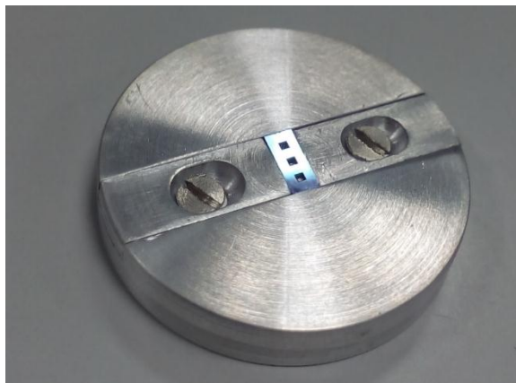
Figure 6.2. Image of the holder used to extend the effective area at which the resist is deposited during the spin-coating process
