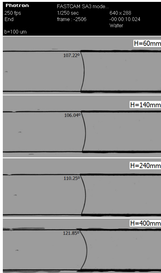
Figure D.1: Curvature interface water-air in a channel of b = 100 \mu\text{m} . We see that the curvature angle increases as the hydrostatic pressure increases. In channel of this depth the capillary forces become more important than in a channel of b = 300 \mu\text{m} , section 5.1.3.
