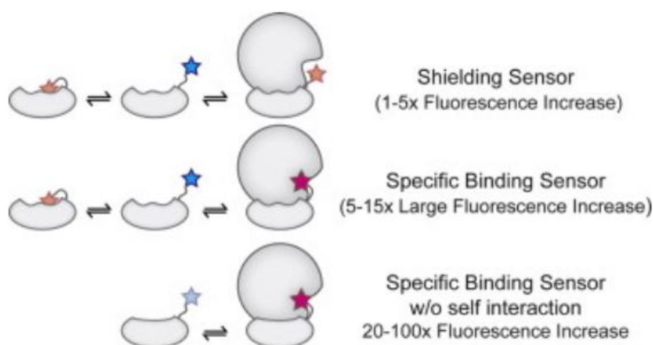
Figure 58. Mechanistic drawing of the three types of reagentless biosensors. The top one describes a sensors that suffers from pre-activation and the fluorophore undergoes shielding upon binding, yielding a small F/F_0 ratio. The middle one describes a sensor that may have some pre-activation but that alleviates this drawback by having a strong fluorescence enhancement due to a fluorophore binding pocket. The bottom scenario describes a sensor that possesses both ideal properties: little self-interaction and specific binding pocket interaction on the analyte. Extracted from Journal of Molecular Biology . 260
