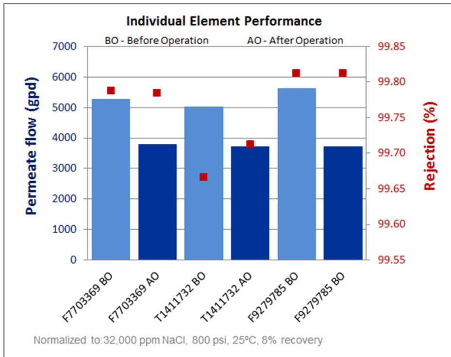
Figure 1.11. Individual element performance before and after the long-term operation
