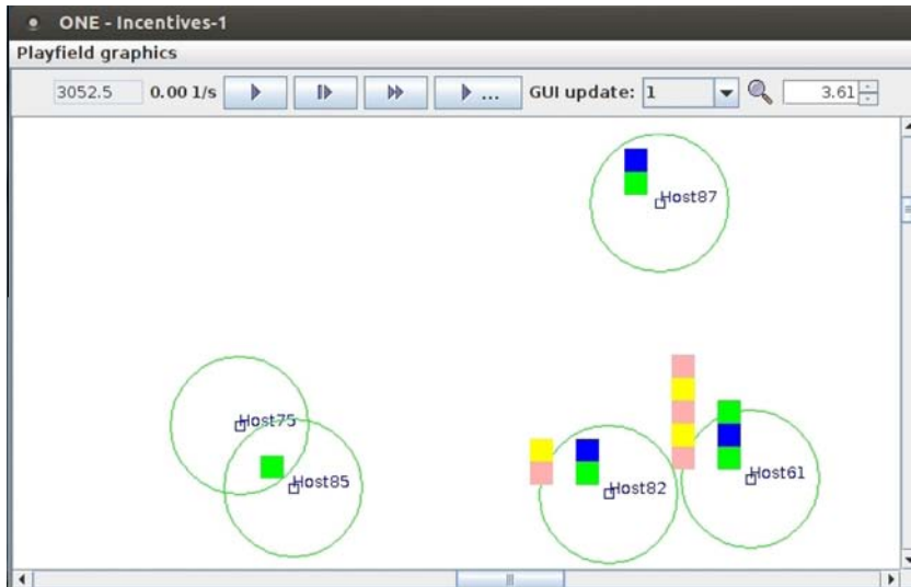
Fig. 5. A snapshot of a simulation. On the upper side, a node carries two messages and waits for an opportunity to forward them. On the left side, one node tries to forward the only message it carries, but the other acts selfishly and rejects the transmission. On the right side, two cooperative nodes just forwarded messages between them, generating some proofs of forwarding.
