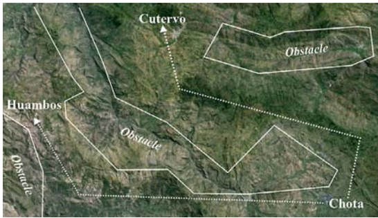
Fig. 12. Map of a scenario of application located in a rural area of Cajamarca (Perú). White lines are natural obstacles approximate limits. Dotted white lines represent the pathways where messages sent from the village of Chota to Cutervo or to Huambos have to be routed through. The size of the area under consideration is 30 \times 30 km.
