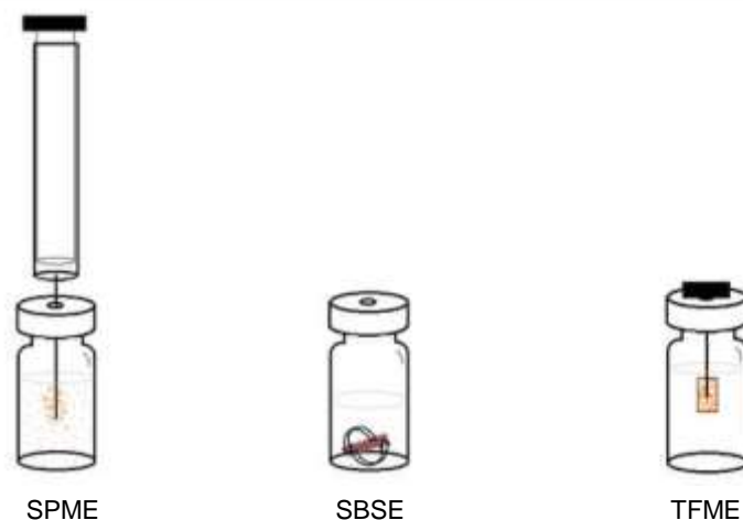
Figure 7: Main solid-phase microextraction techniques [158].
