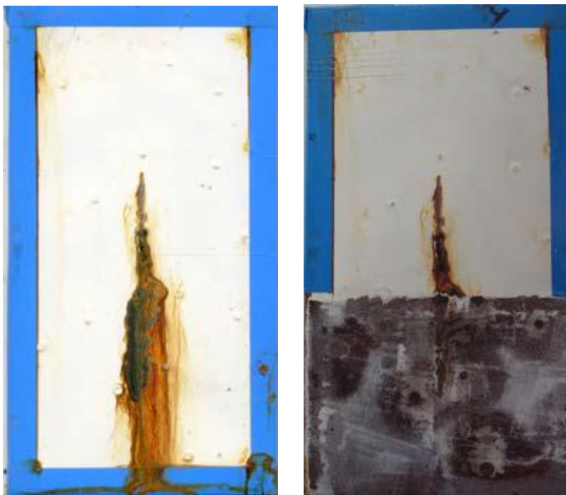
Figure 8.4. Photograph of the Reference panel after 1440 hours in the salt spray chamber: initial stage (a) and one half panel withor coating.
