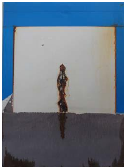
Figure 7.8. Photograph of the 6% Pigment C panel after 1.100 hours in the salt spray chamber.
