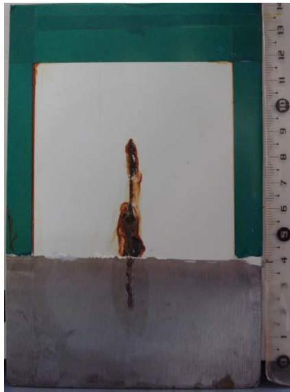
Figure 7.9. Photograph of the 8% Pigment C panel after 1.100 hours in the salt spray chamber.
