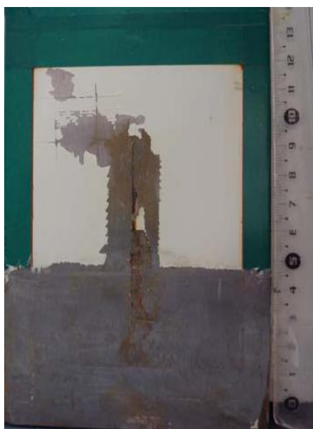
Figure 6.3. Photograph of the Reference panel after 641 hours in the salt spray chamber.
