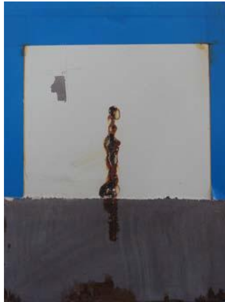
Figure 7.10. Photograph of the 10% Pigment C panel after 1.000 hours in the salt spray chamber.
