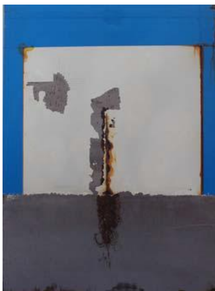
Figure 7.7. Photograph of the Reference panel after 1.100 hours in the salt spray chamber.
