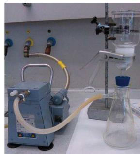
**Figure 3.8.** Experimental set-up for TiO<sub>2</sub> fixation by heat and pressure treatment.
