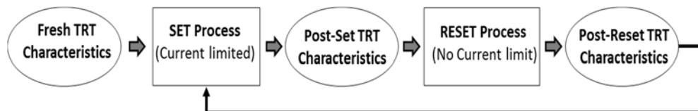
Figure 2-11: Stress-measurement sequence designed to analyze the the gate current contribution at HRS in MOSFETs.
