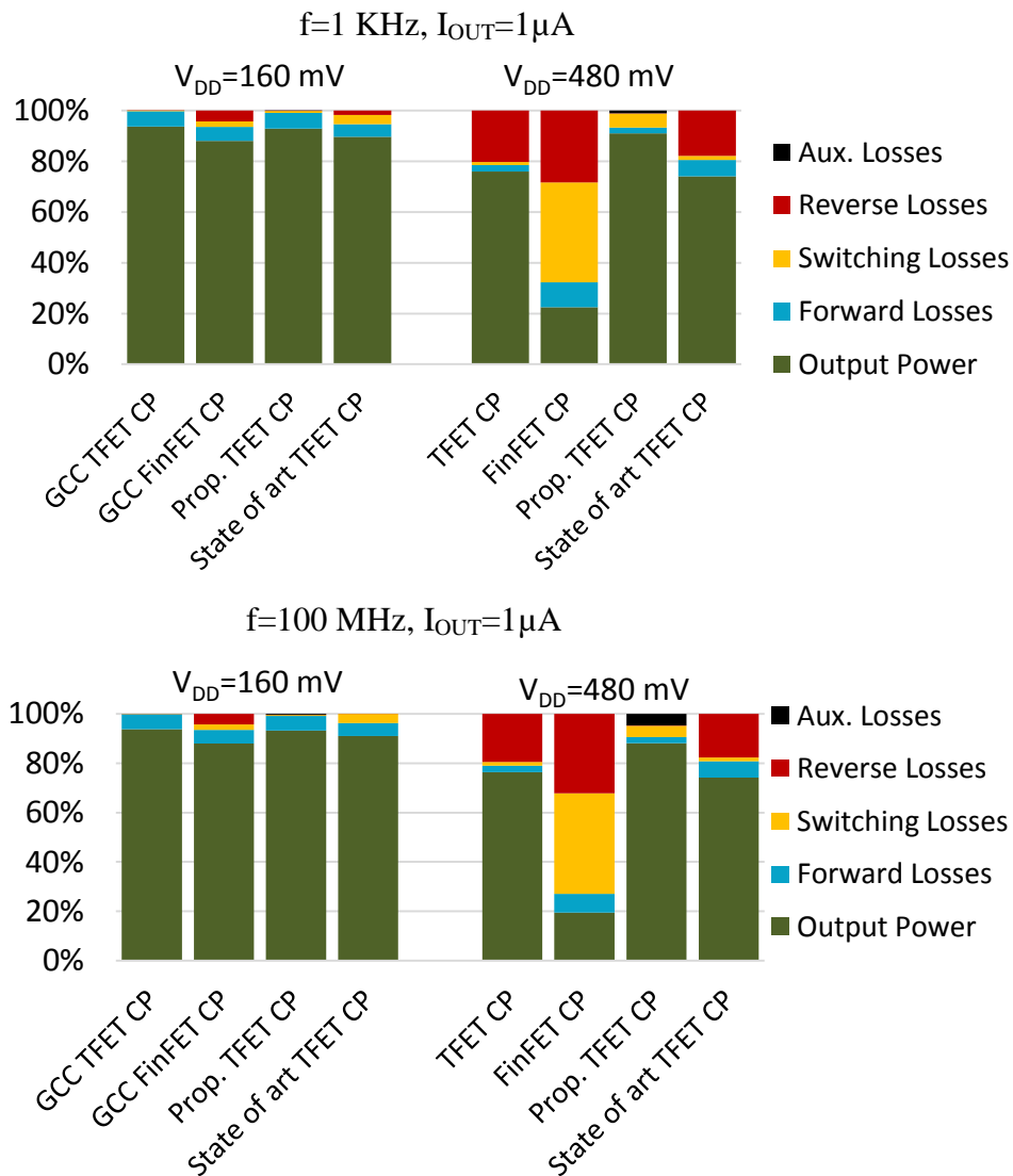
Fig. 5.13 Distribution of power losses in the charge pumps for clock frequency of 1\ \text{kHz} and 100\ \text{MHz} and load of 1\ \mu\text{A} .
