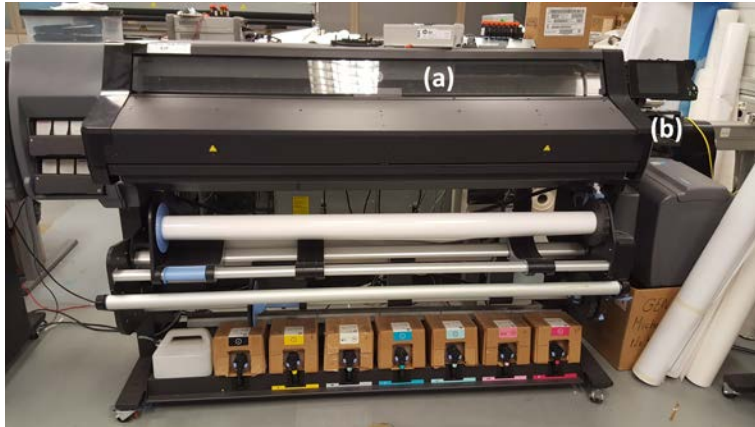
Figure 3.1: The printer (HP Latex 560) used for the tests. (a) Printing area and (b) spittoon marks the regions where samples were installed during first and second tests, respectively.
