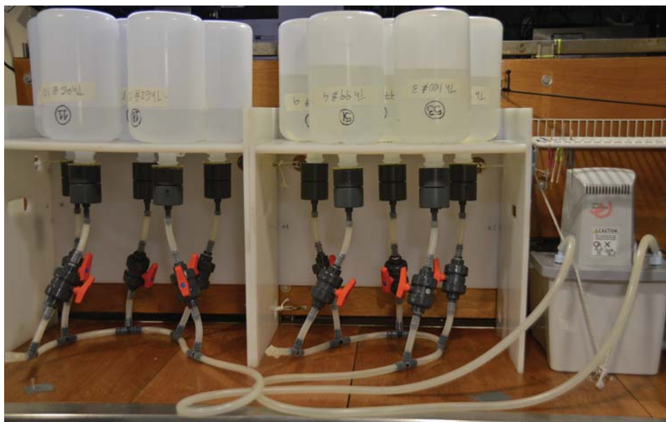
Figure 2.1: Filtration system for ^{234}\text{Th} with 4-L bottles connected to an Eyela aspirator vacuum pump.
