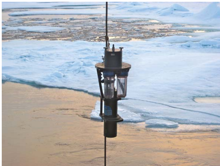
Figure 2.5: In situ pump employed during the ANT-XXVIII/3 and ARK-XXVII/3 expeditions (Chapters 3 and 4).
