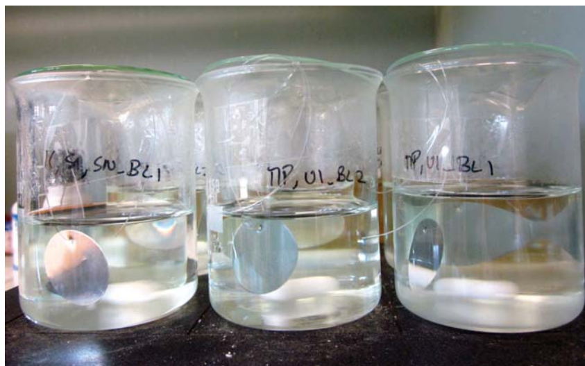
Figure 2.3: Auto-deposition of Po isotopes onto silver discs using a hot plate that allows temperature and stirring control.
