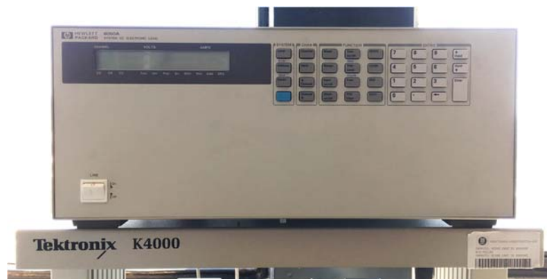
Fig. A.9. Electronic load from HP composed of mainframe model 6050A and three power modules model 60504B with a maximum power, voltage and current of 600 W, 60 V, and 120 A, respectively, per module.
