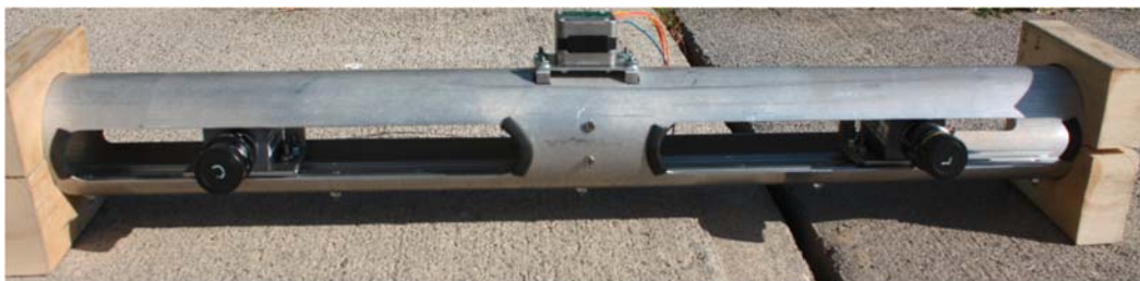
FIGURE 2.6: Stereo camera, with variable geometry, from (Fanto, 2012).
