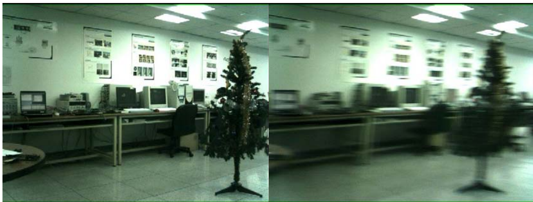
FIGURE 2.3: Left: static image for reference. Right: same office scene captured with movement, showcasing artifacts induced by rolling shutter: not only is the image is blurred due movement, but the straight lines are distorted presenting a slight curvature.
