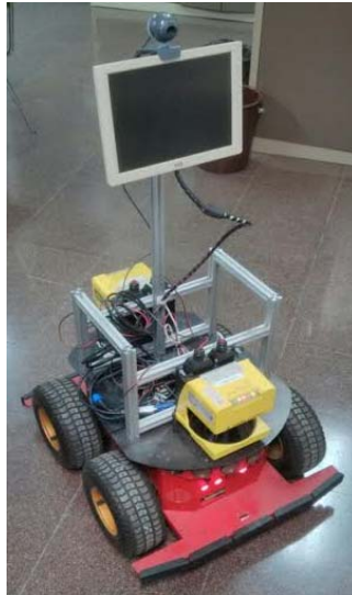
FIGURE 5.10: Robotic platform Pioneer AT3 with a test webcam and laser range finders.
