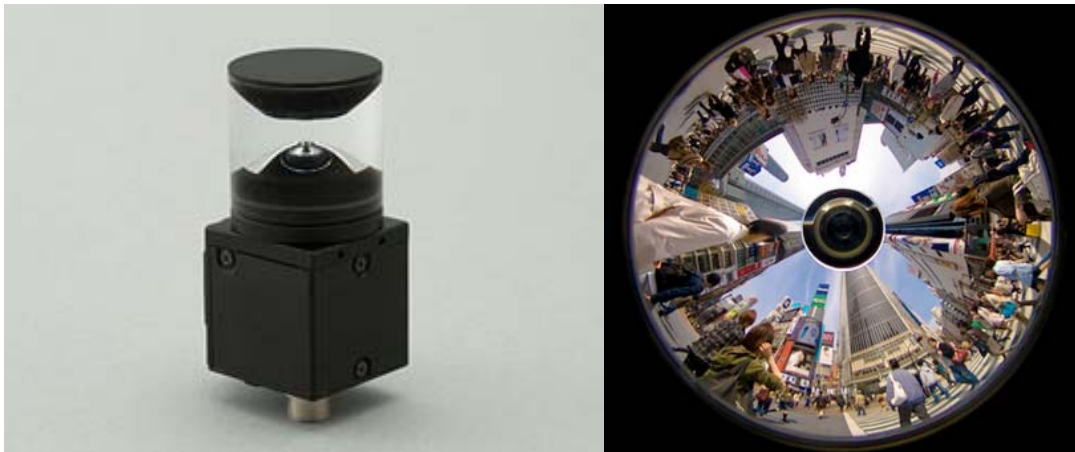
FIGURE 2.5: Omnidirectional camera (courtesy of Olympus). Left: Camera sensor with mirrors to project 360° around yaw axis. Right: Sample shot from an omnidirectional camera.
