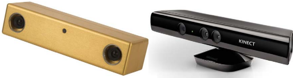
FIGURE 2.7: Left: stereo based RGB-D camera (courtesy of PointGrey). Right: Kinect, with its IR emitter, IR depth camera, and colour camera all visible (courtesy of Microsoft).
