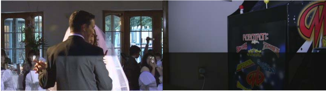
FIGURE 2.4: Rolling shutter in a CMOS sensor with non-continuous lightning. Left: effects of a camera flash from another device in a professional CMOS camera. Right: image taken under a fluorescent light with incorrect capture synchronization timing in the camera.
