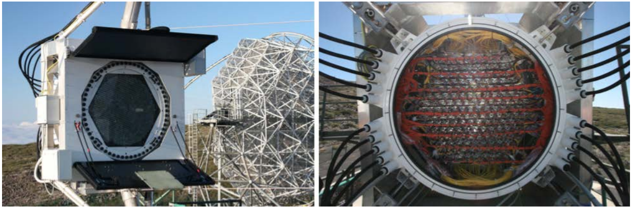
Figure 2.19: Front ( left ) and back side ( right ) of the MAGIC II camera. The current MAGIC I camera is a clone of this.
