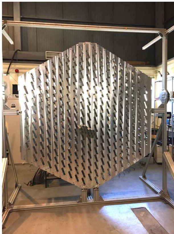
Figure 10.4: Metallic structure holder for the modules of the LST. The module are placed in each hole. In the center, two modules are connected, which have attached the light guides.
