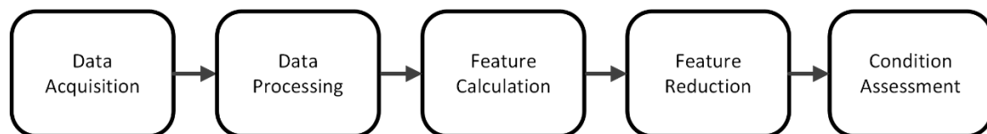
Fig. 1.1.1 Five main stages in a knowledge-based CBM program to facilitate the maintenance decision making.
