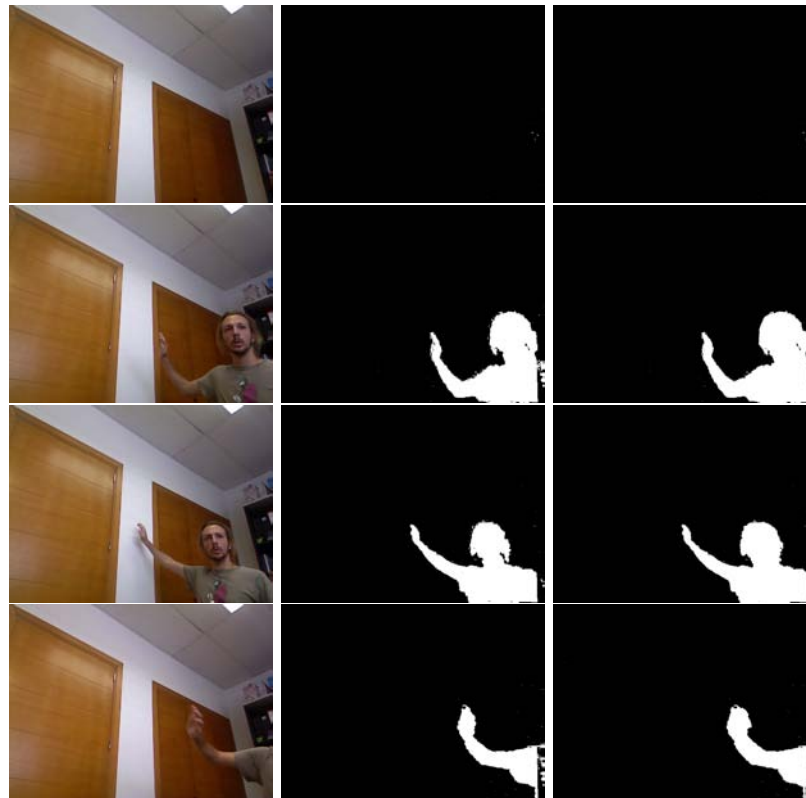
Fig. 4.23: Results of Shadow sequence: Left column corresponds to color images used as reference, right column is the result of the algorithm considering undefined pixels as foreground ( GSM_{UF} ) and the column at the center is the result of the algorithm considering undefined pixels as background ( GSM_{UB} ).
