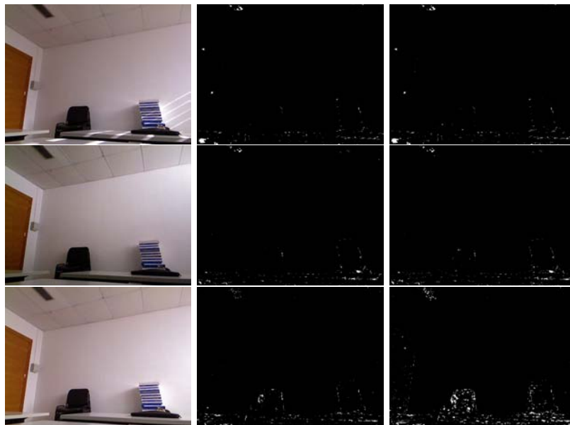
Fig. 4.20: Results of Time Of Day sequence: Left column corresponds to color images used as reference, right column is the result of the algorithm considering undefined pixels as foreground ( GSM_{UF} ) and the column at the center is the result of the algorithm considering undefined pixels as background ( GSM_{UB} ).
