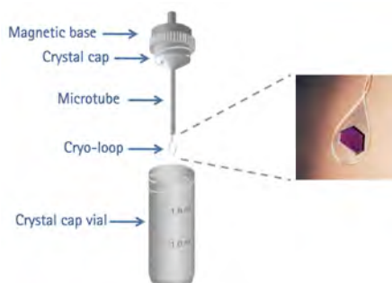
Figure 2-8. Diagram of a cryo-crystallography system (left) and a cryo-loop with a crystal mounted (right)
