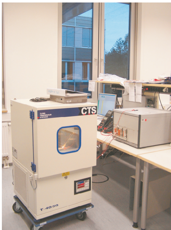
Figure F.3: Measurement setup for battery characterization including a climate chamber.
