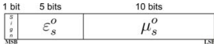
Figure 3.11: Structure of the \Delta_s^o Sub-marker.
