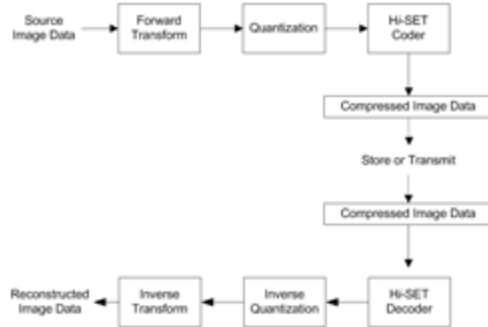
Figure 3.1: General block diagram of a generic compressor that uses H_i -SET for encoding and decoding.
