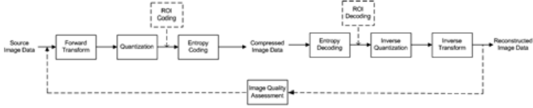
Figure 1.2: General Block Diagram for an image compression system.
