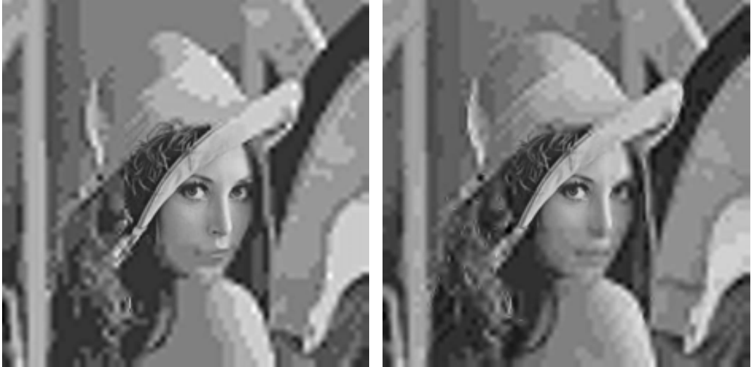
(a) MaxShift method in JPEG2000 coder, (b) MaxShift method in Hi-SET coder, 0.34 bpp. 0.34 bpp.
