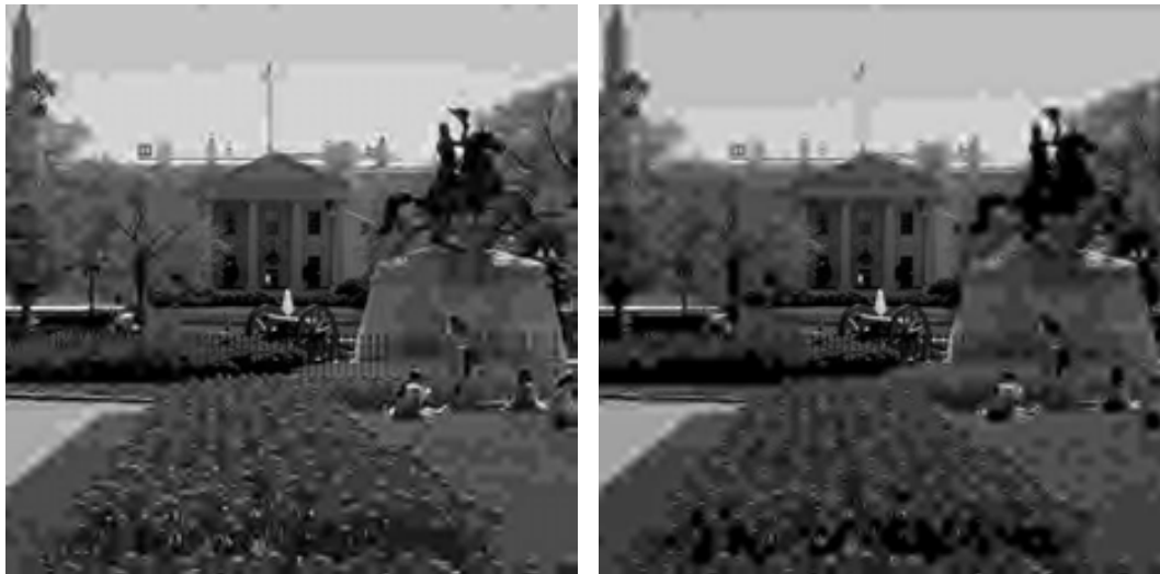
(a) MaxShift method in JPEG2000 coder, (b) MaxShift method in H \dot{i} -SET coder, 0.42 bpp.
