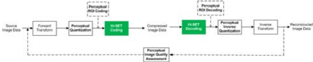
Figure 3.2: General block diagram for the proposed perceptual image compression system. The H_i -SET compression algorithm is indicated by the green blocks.
