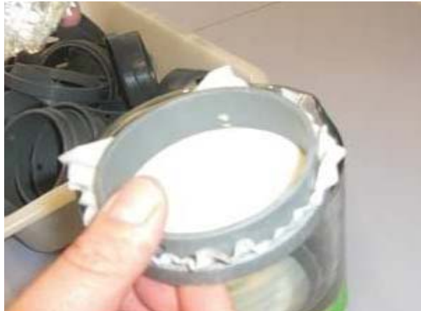
Figure 7: SPATT-discs filled with DIAON ® HP20 styrene divinylbenzene resin (Mitsubishi Chemical Corporation). Photo: IRTA (2010).
