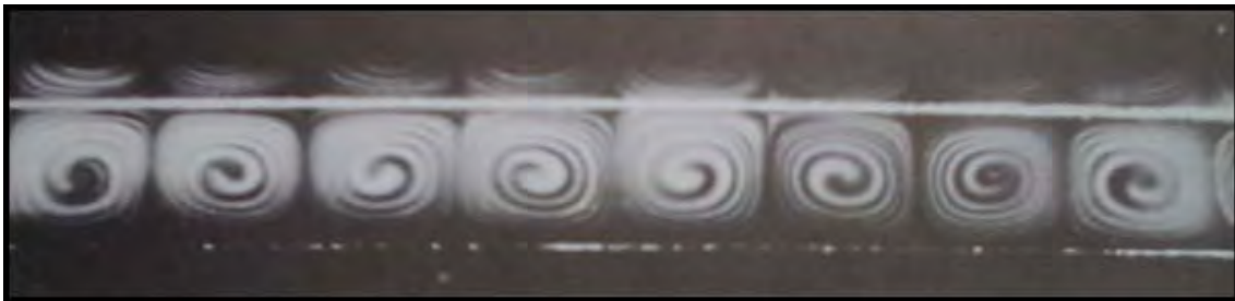
Figure 3.1: Cross section of convection cells in channel flow; Ra = 4.16 \times 10^3 , Re = 8.3 . (Tritton 1999).
