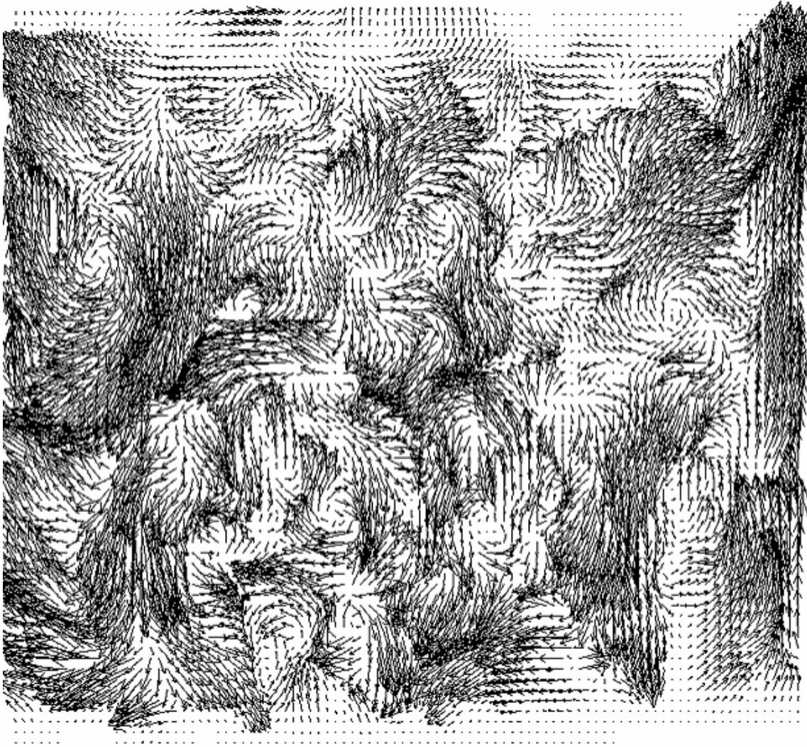
Fig A3.5: High resolution velocity map of a vertical grid stirred decaying flow in the Trondheim rotating facility, Ro = 1.3 and Ri = 0.002 at 2 seconds after the grid drop.
