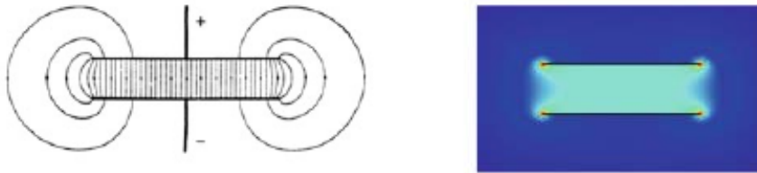
Fig. 11: As shown in the theoretical model, plate electrodes are able to produce a more homogeneous Electrical field (E) (Kee et al., 2011)
