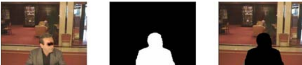
Figure 3.4: Example of an application where we can segment an object (person) in the foreground of a scene, since the background is always the same. Therefore only the pixels in the background might be considered in the channel normalisation process.
