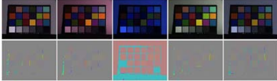
Figure 3.6: The non-iterative comprehensive normalisation for five images of the same scene under five different illuminants, where the sensor is calibrated for the illuminant of the first image.
