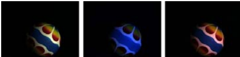
Figure 2.9: Three images of the same scene under three different illuminants, where the camera is calibrated for the illuminant of the first image.
