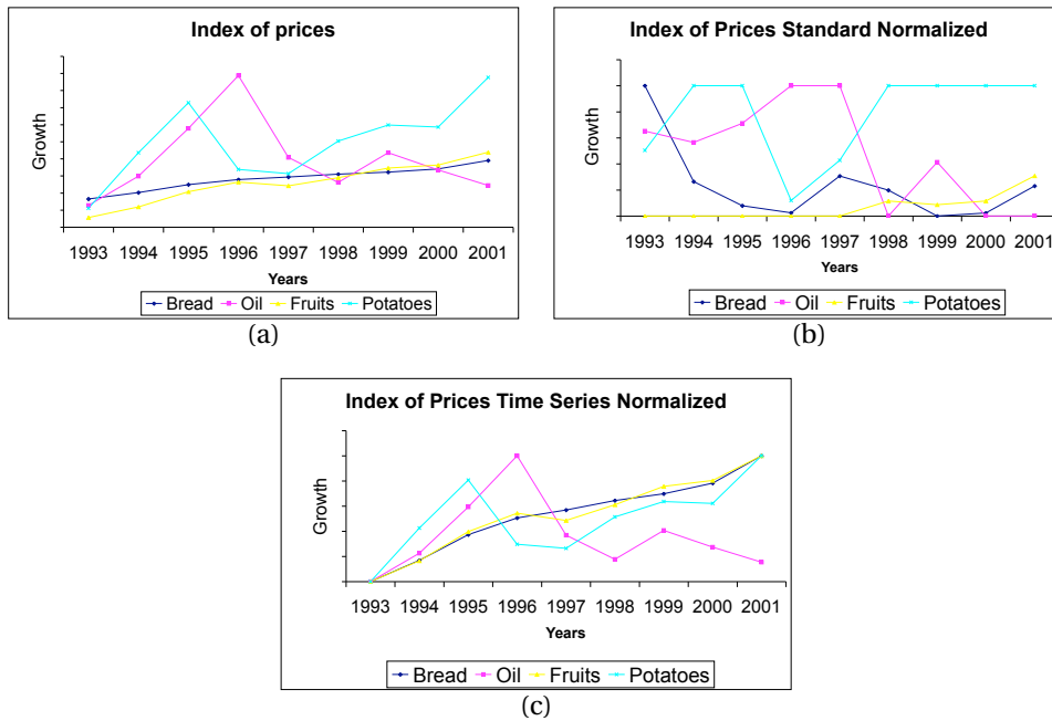
Figure 6.2: Graphical representation of the effects of time series normalization, (a) represents the original data without normalization, (b) represents normalized data with independent normalization, (c) represents normalized data with time series normalization.
