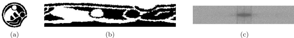
Figure 2.4: Example of the generic Fourier descriptor. (a) An original logo image; (b) polar-raster sampled image plotted in Cartesian space; (c) Fourier spectra of (b); (reprinted from [ZL02]).
