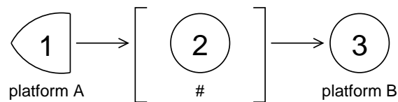
Figure 3.6: Example itinerary with a discoverer node and a dynamically located node.
