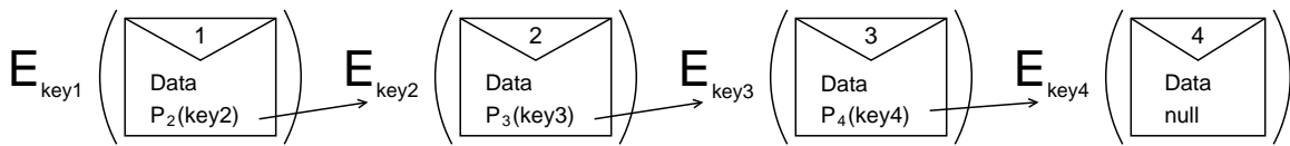
Figure 4.1: Representation of a chain of digital envelopes.
