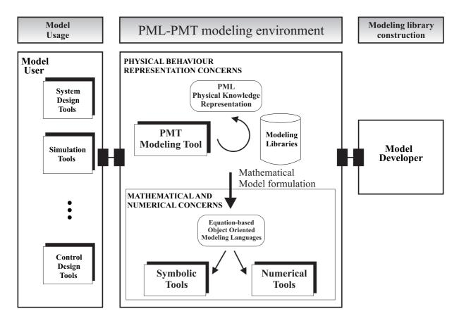
Figure 1.8. Schematic representation of the PML modeling environment architecture.
