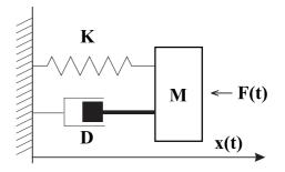
Figure 1.3. Mechanical system with a mass, a spring and a damper. M, D and K are the system parameters, F(t) is an external force applied to the system and x(t) represents the mass position.
