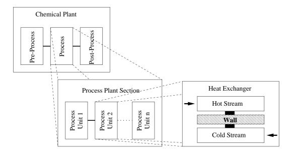
Figure 1.5. Structured modeling of chemical process. The models of the process units are successively connected according to the system topology.
