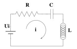
Figure 1.2. Electrical RLC circuit. R, L and C are system parameters,  $U_i$  is the voltage input signal and i is the electrical current.
