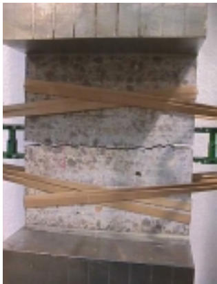
Figure 3.20. Failure plane of the 50 mm thick panel
