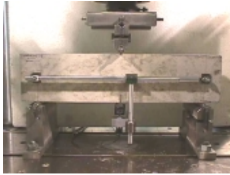
Figure 3.28. Flexure test set-up
