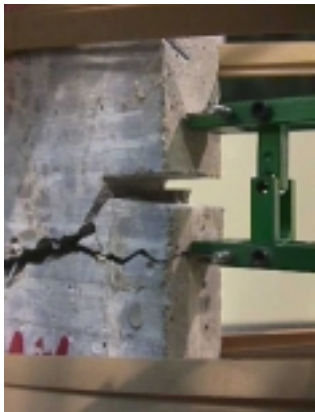
Figure 3.21. Example of unexpected failure in some 25 mm thick panels
