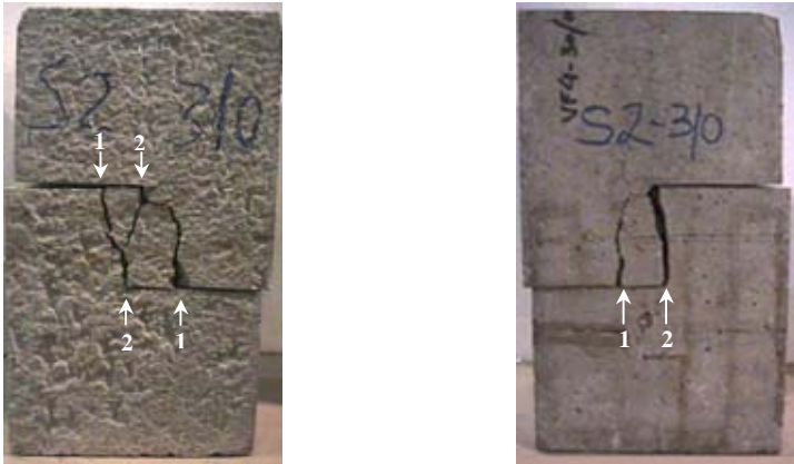
Figure 4.8. Typical failure modes for plain NSC (both sides of the same specimen)
