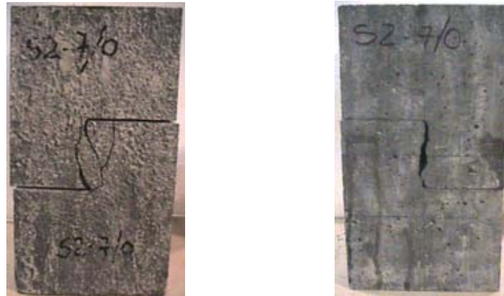
Figure 4.9. Typical failure mode for plain HSC (both sides of the same specimen)
