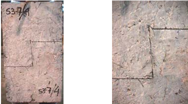
Figure 4.11. Typical failure mode for HS-SFRC (same specimen, closer view on the right)
