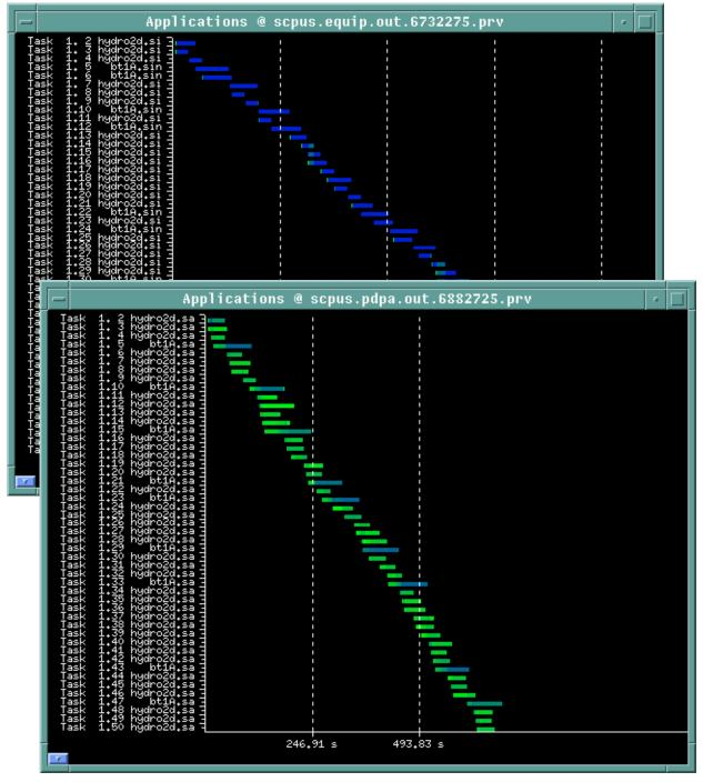
Figure 5.20: Workload 2, processor allocation decided by Equipartiton and PDPA (M.L=2, load=100%)
