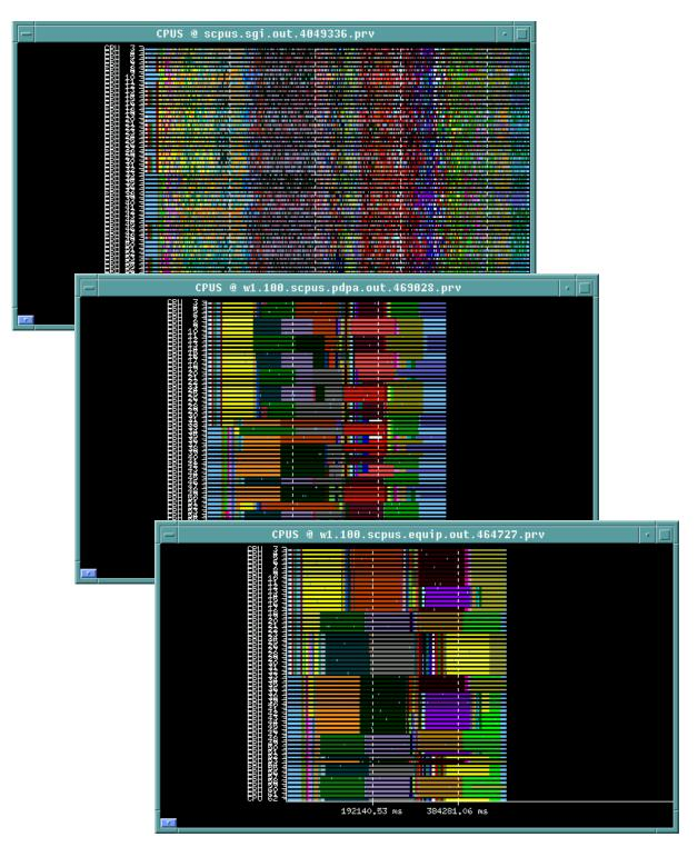
Figure 5.13: Execution views for workload 1 under IRIX, PDPA, and Equipartition (load=100%)
