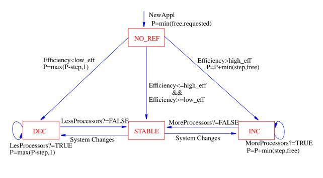
Figure 5.1: PDPA: Application state diagram
