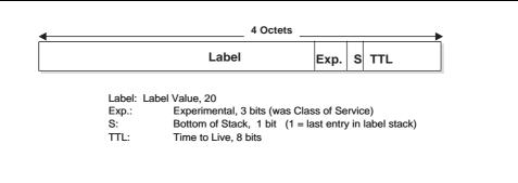
evant on a single link, between adjacent LSRs. Figure 1.3 presents the fields of an MPLS "shim" header.
