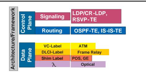
Figure 1.1 Control and Data plane components
