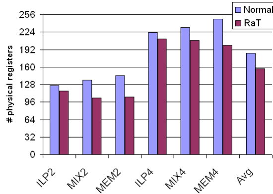
Figure 3.27: Average physical registers used per cycle between normal and runahead threads
