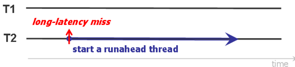
Figure 3.1: A runahead thread is started when a long-latency load is detected
