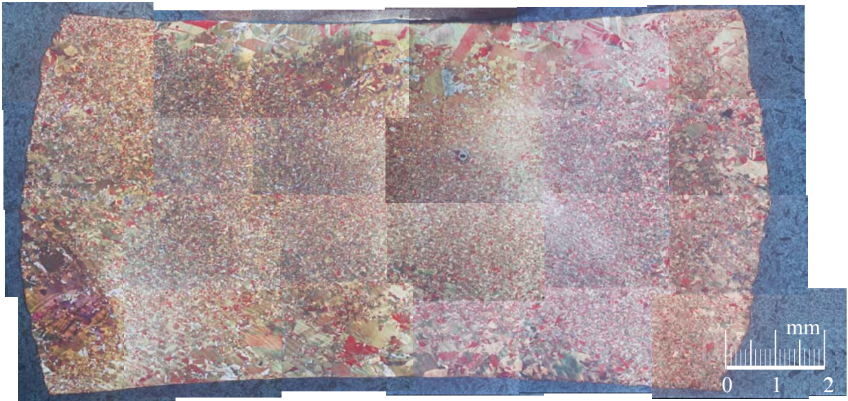
Fig. F.3. Macrograph of compressed Cu B test cylinder after 750°C, 0.3s -1 and \epsilon = 0.8 .
