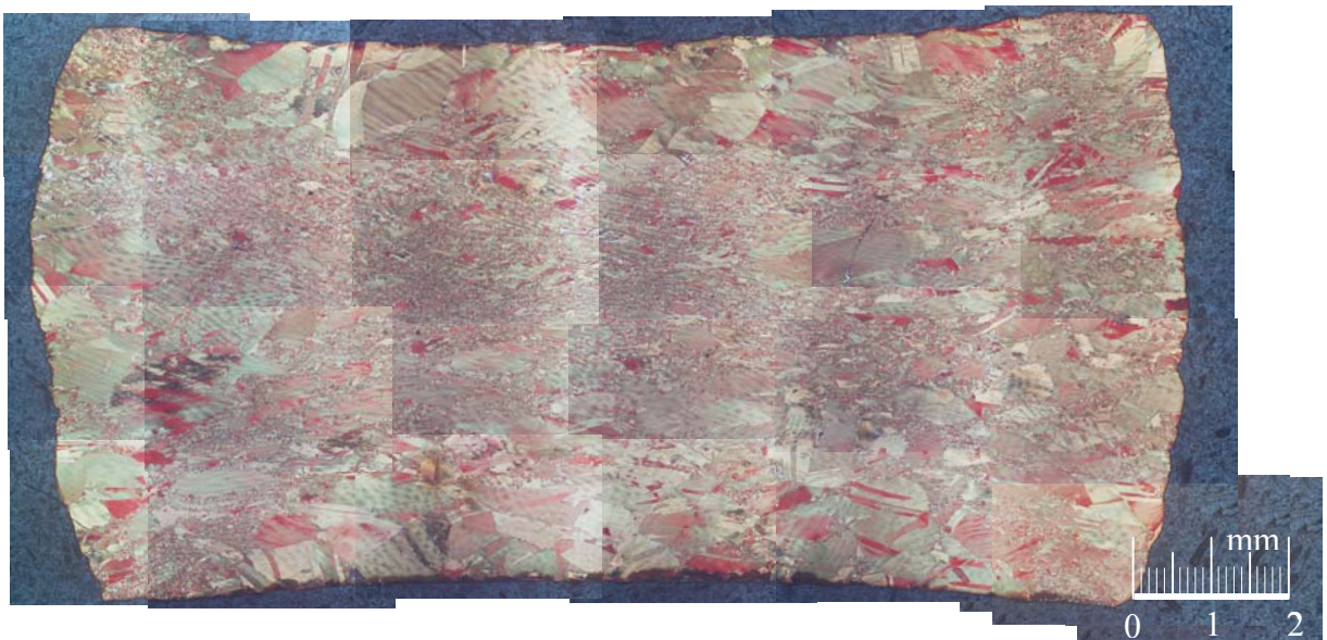
Fig. F.2. Macrograph of compressed Cu B test cylinder after 700°C, 0.3s^{-1} and \varepsilon = 0.8 .
