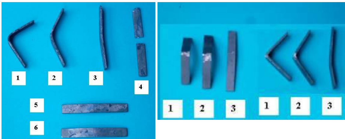
Figure 6.11: Influence of the exposure to air at 1500°C air on the ductility of Cr and Cr-35Re
