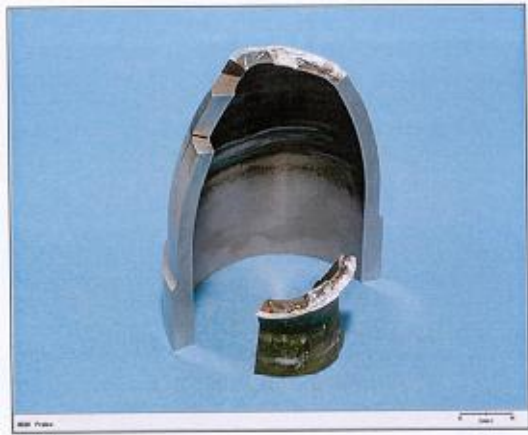
Fig 1.12: Global appearance of the combustion chamber. The green surface consists of chromium oxides. The fracture near the throat is the most evident failure point of the chamber.
