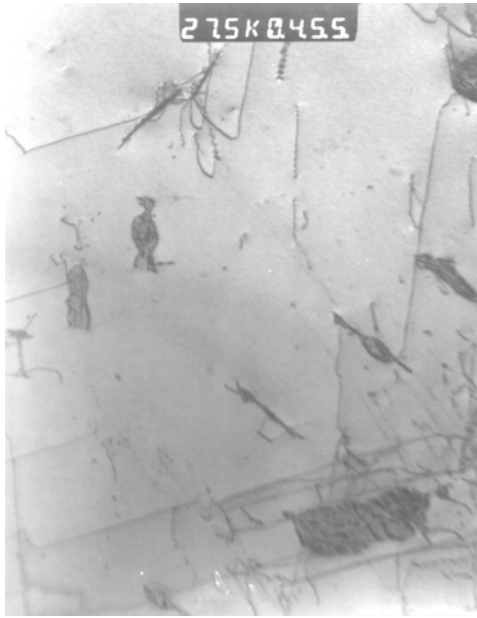
Figure 1.18a: Transmission electron Microscope image of the microstructure of the as manufactured material. There is a relatively high dislocation density, indicating its non fully recrystallised condition but no precipitation at dislocation borders, generally in the form of dark shadows, indicating the high purity of the material.
