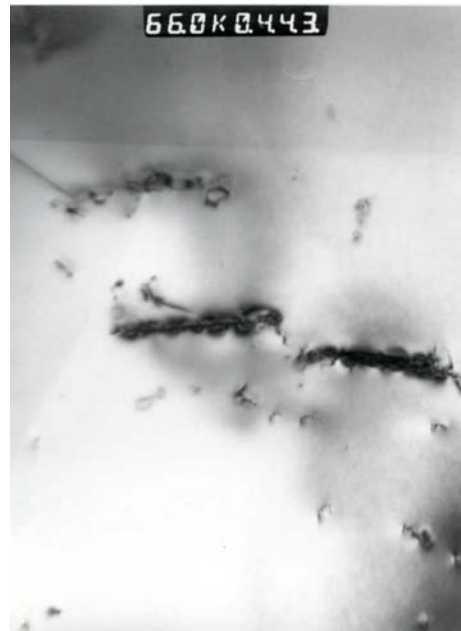
Figure 1.18b: Precipitation of nitrides at dislocation borders made evident by transmission electron microscopy (dark areas). The low dislocation density is a result of the high recrystallisation of the material. Nitrides and carbides surround remaining dislocations. These are the main responsible for the material brittleness.
