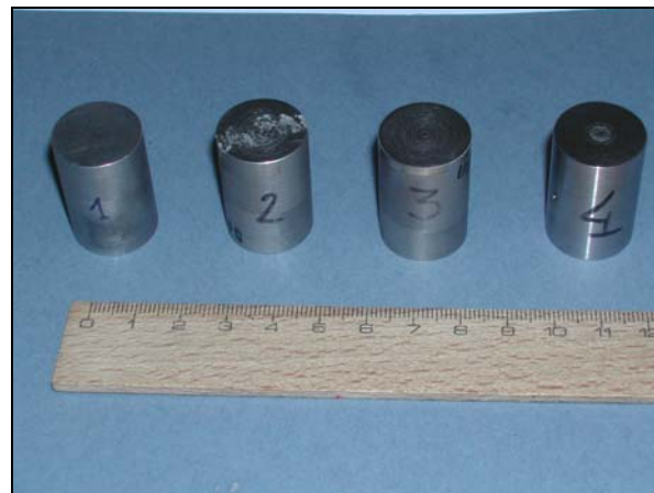
Figure 8.2: Samples used for the measurement of the thermal properties
