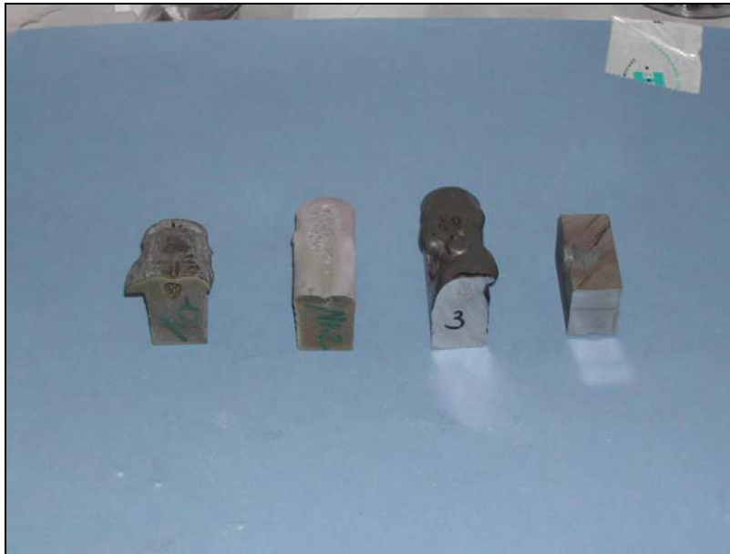
Figure 8.7 > Samples used for the measurement of the electrical conductivity
