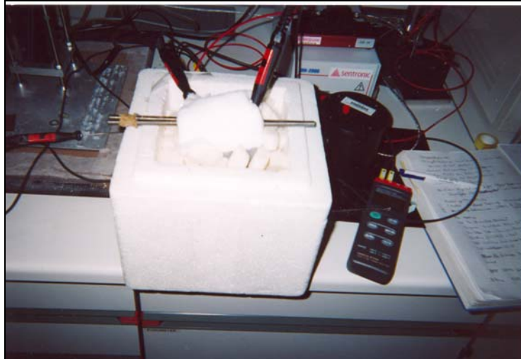
Figure 8.12: Temperature recording to measure the equilibrium temperature
