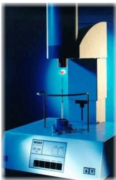
Figure 8.20: Laser flash DSC apparatus 404 C Pegasus used in the study
