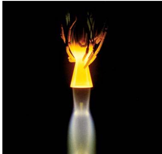
Figure 1.11b: Vacuum firing test of a 400N combustion chamber. Source Astrium.
