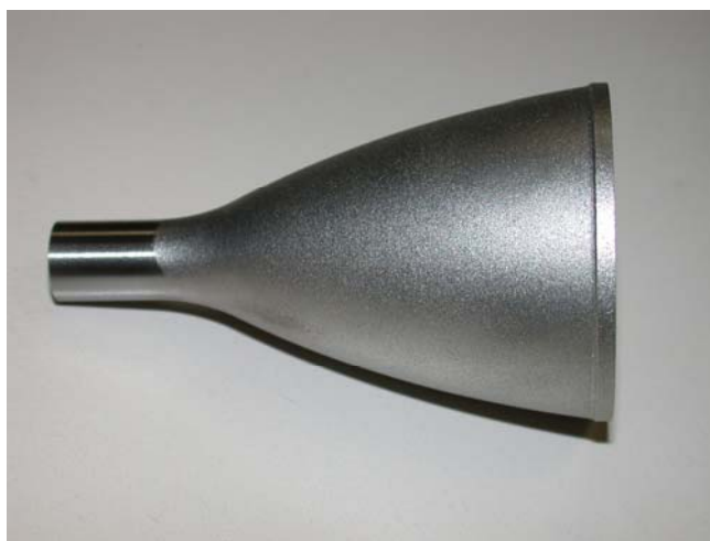
Figure 10.1: First Cr-35Re satellite thruster engine for pre-qualification.
