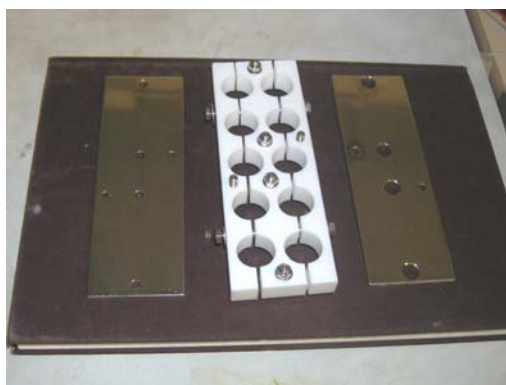
Figure 3.14 : Teflon moulds with stainless steel covers used to manufacture the composite scaffolds
