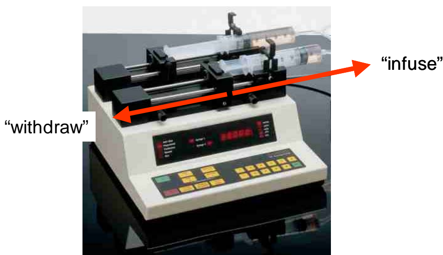
Figure 6.1: Photograph of the syringe pump used for the dynamic cell seeding with MSC cells.
