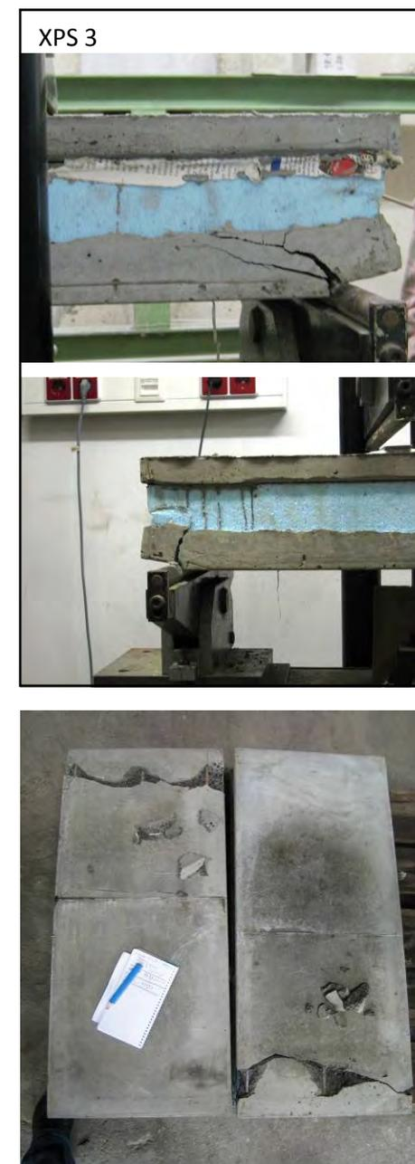
SANDWICH PANEL WITH EXTRUDED POLYSTYRENE CORE
