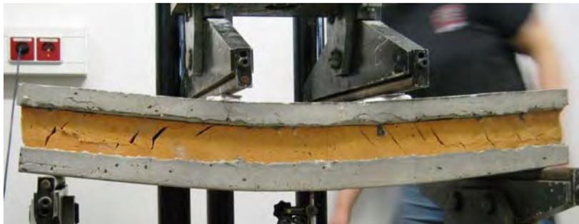
The top layer was suffering compression and now has an added bending effort, while the bottom layer adds new bending to a tensile effort. Inner forces increase but the effective section is now thinner.
