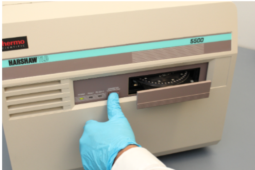
Figure 6.2: HARSHAW reader and wheel at the start of the reading process
