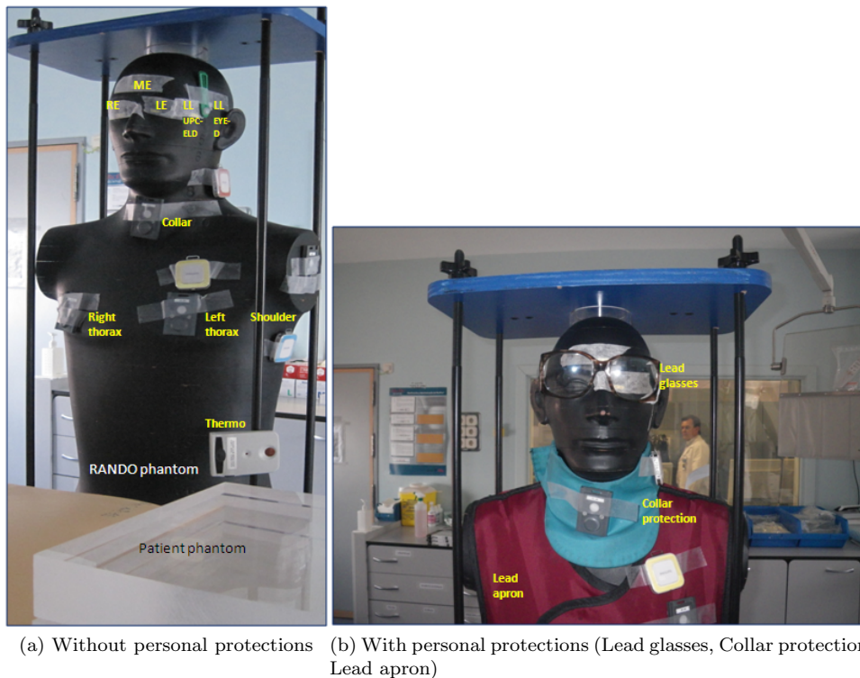
Figure 11.3: Positioning of the dosimeters (EYE-D, UPC-ELD, UPC-WBD, active dosimeters) on the RANDO phantom
