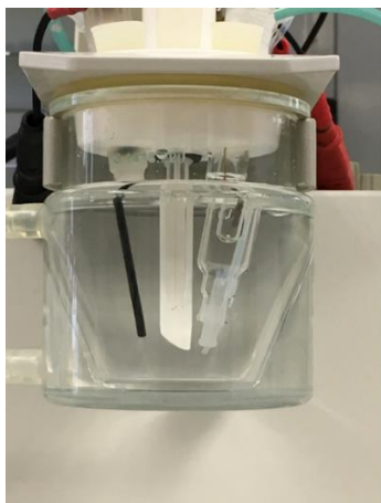
Figure 2-12: Voltammetric cell with stirrer, double-junction Ag/AgCl/3mol L -1 KCl, Metrohm Hanging Mercury Drop (HMDE) and Glassy carbon were used as reference, working and auxiliary electrodes, respectively.
