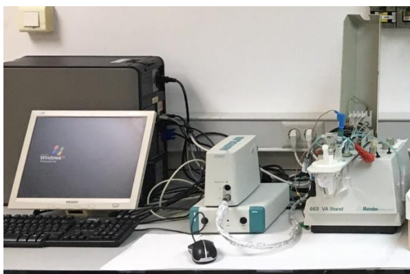
Figure 2-13: Equipment used for the measurements including glass cell, Autolab potentiostat and Metrohm polarographic Stand.
