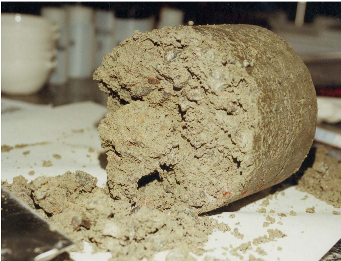
Figure 3.37: A backfill specimen after being hydrated during 100 days with distilled water. When the backfill was extruded from the cylindrical mould, the water content was measured in five different slices (CIEMAT, 2002).
