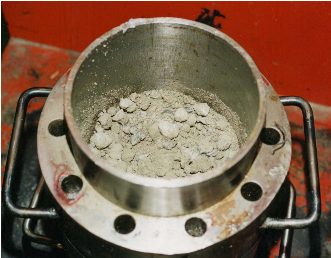
Figure 3.31: Backfill within CIEMAT's metallic mould before to its static compaction. A water uptake test with distilled water was performed in this specimen after compaction (CIEMAT, 2002).
