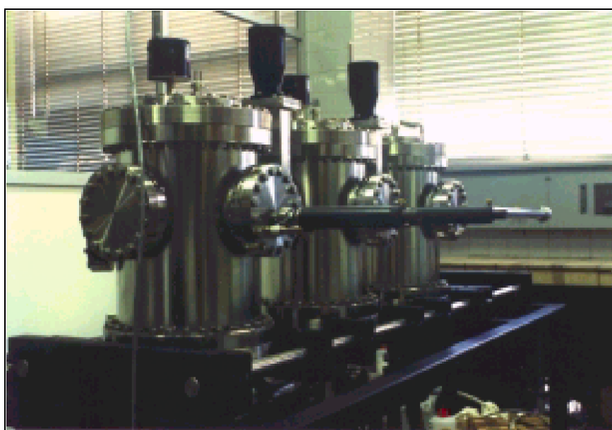
Figure 2.2. Picture of the Hot-wire CVD chamber, situated in the Department of Applied Physics and Optics, Universitat de Barcelona
