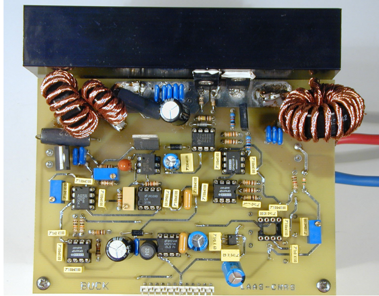
Fig.5.5 A 100 W BIF converter-based G-yrator used in the gyrators paralleling
