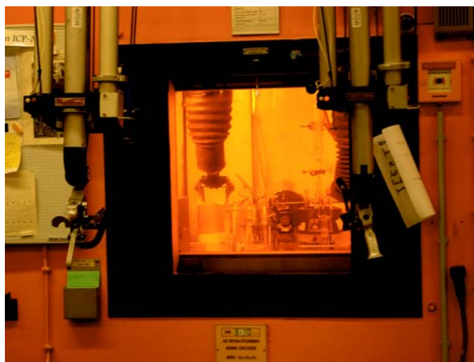
Figure 9: Hot-cell facility installed at EC-JRC-ITU.
