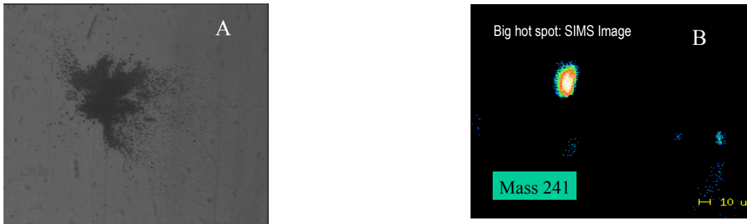
Figure 2. A. Autoradiography of the Am particle found in the layer 26-28 cm. B. SIMS image of the particle.
