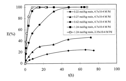
FIGURE 1. Effect of extractant content in the resin (expressed in mol/kg dry XAD2 resin) on extraction kinetics of Pd(II) by XAD2/DEHTPA resins. Experimental conditions: mass of resin 0.1g, volume of aqueous phase 20 ml, HCl 0.5 M and initial Pd(II) concentration 2.35x10<sup>-4</sup> M or 4.7x10<sup>-4</sup> M.
