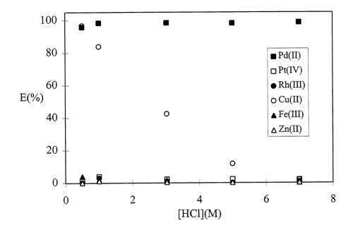
FIGURE 6. Effect of HCl concentration on percentage extraction of heavy metals. Experimental conditions: mass of resin 0.1g, volume of aqueous phase 20 ml, DEHTPA concentration 1.24 mol/kg dry XAD2 resin, initial Pd(II) concentration  $4.7 \times 10^{-4}$  M and shaking time 16 h.
