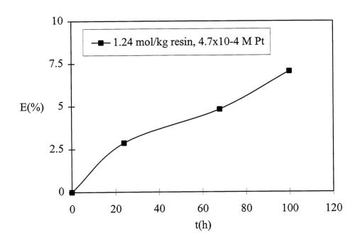
FIGURE 2. Extraction kinetics of Pt(IV) by XAD2/DEHTPA resins. Experimental conditions: mass of resin 0.1g, volume of aqueous phase 20 ml, DEHTPA concentration 1.24 mol/kg dry XAD2 resin, HCl 0.5 M and initial Pt(IV) concentration  $4.7 \times 10^{-4}$  M.
