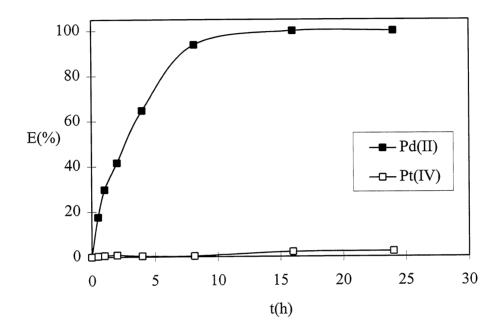
FIGURE 3. Percent extraction of Pd(II) and Pt(IV) against contact time. Experimental conditions: mass of resin 0.1g, volume of aqueous phase 20 ml, DEHTPA concentration 1.24 mol/kg dry XAD2 resin, HCl 0.5 M and initial metal concentrations  $[Pd]_i=[Pt]_i=4.7x10^{-4} M$ .
