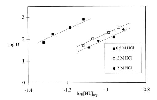
FIGURE 5. Effect of free HL concentration (expressed in mol/kg dry impregnated resin) on the distribution ratio of Pd(II). Solid lines were plotted taking into account slope 4. Experimental conditions: the same as those in Figure 4.
