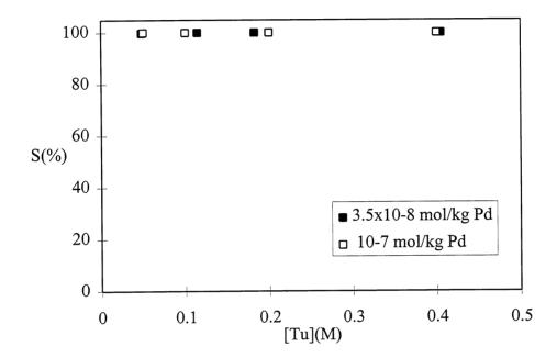
FIGURE 7. Effect of thiourea concentration in HCl 1 M medium on the percent stripping of Pd(II) loaded with XAD2/DEHTPA resins. Experimental conditions: mass of resin 0.1 g, volume of the stripping aqueous phase 10 ml, variable metal content in the resin (expressed in mol/kg dry impregnated resin) and stripping shaking time 24h.
