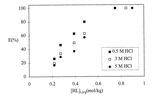
FIGURE 4. Effect of the initial HL concentration on the resin ([HL]<sub>i,org</sub>, expressed in mol/kg dry XAD2 resin) on percent extraction of Pd(II) with XAD2/DEHTPA resins. Experimental conditions: mass of resin 0.1g, volume of aqueous phase 20 ml, initial Pd(II) concentration  $4.7 \times 10^{-4}$  M and shaking time 60 h.
