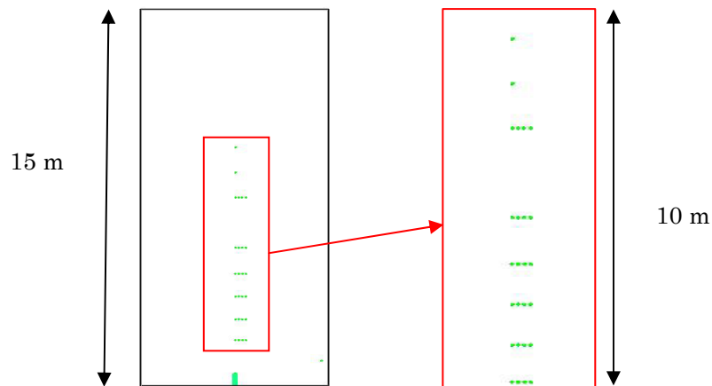
Figure 6.5 Position of the thermocouples on the FDS simulations
