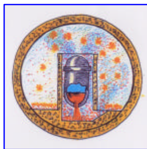
f) Containment direct heating
