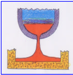
e) Expulsion of melt corium
