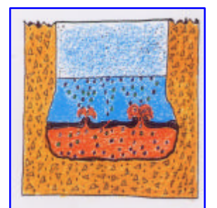
h) Corium-concrete interaction
