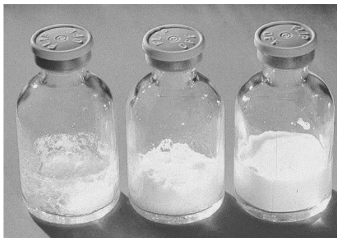
Figure 3.11. Freeze-dried vials with: total collapse (left) and partial collapse (center) and with no evidence of collapse (right). Copied from reference 34 .
