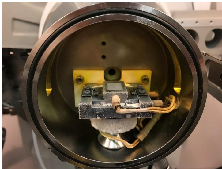
Figure 7.2. Real picture of frozen sample at -50°C inside the LT-XRPD chamber.
