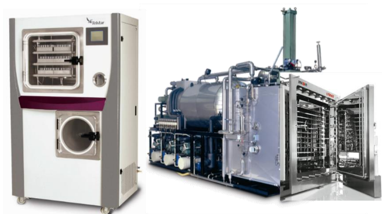
Figure 6.2. Representation of a Lyobeta20 freeze-dryer (left) and industrial freeze-dryer (right). Lyobeta20 freeze-dryer is a model example which does not contain the sample thief in the front door.
